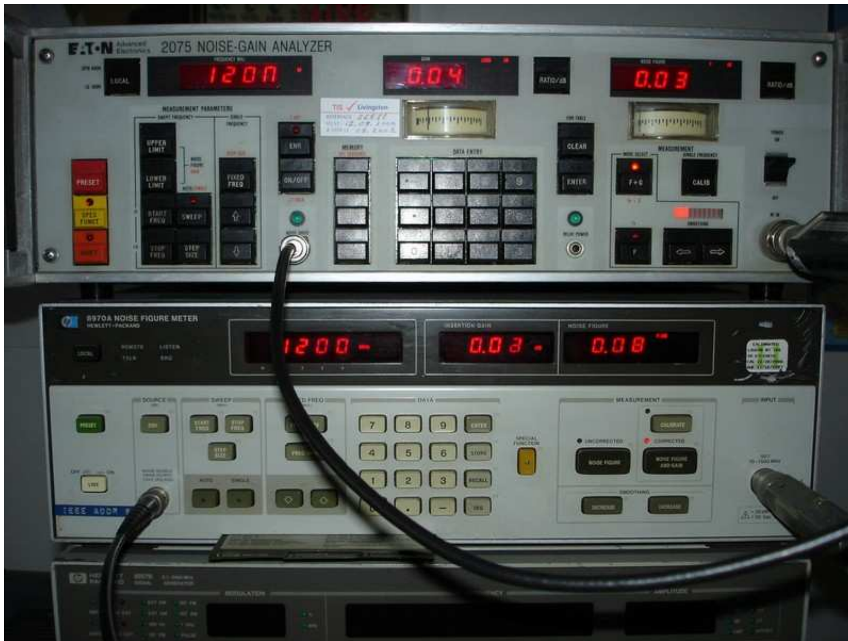
F5DQK January 2009 part 1/4 Eaton 275a and HP/ Agilent 8970a noise/gain analyser
